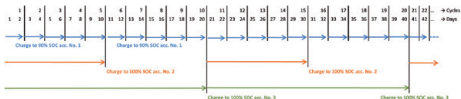
Fig. 7-5: Battery cycles ranging longer than one day
